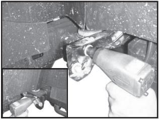
5. Remove two bolts from each side (unplug fog lights if equipped) and set bumper aside.
